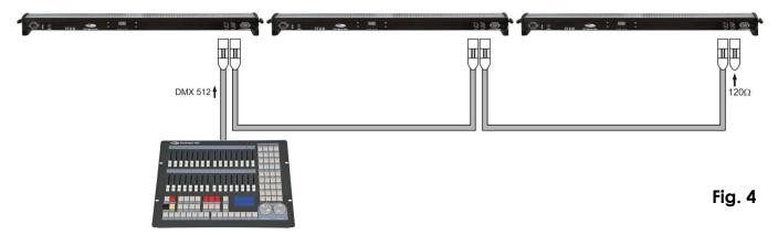
Note: Link all cables before connecting electric power
